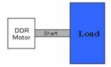
In this model, consider that the shaft has torsional compliance giving it the characteristic of a spring. The motor inertia coupled to the load inertia by a spring will give rise to a mechanical resonance. The goal of the DDR system designer is to make the resonate frequency as high as possible.
